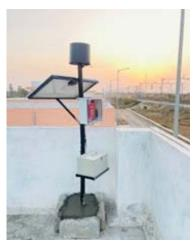
Introducing a cutting-edge Online Multi-parameter Air Quality Monitoring System. This system tracks key air quality indicators including CO, SO2, NO, NO2, O3, CO2, CS2, H2S, and TVOC, among others. It is versatile, suitable for monitoring air quality in diverse settings such as industrial production sites, tunnel traffic environments, and urban areas. The system enhances the collection and
